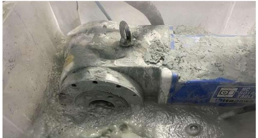
Gear oil in a state where the seal of the standard NC rotary table is worn and cutting water has entered
